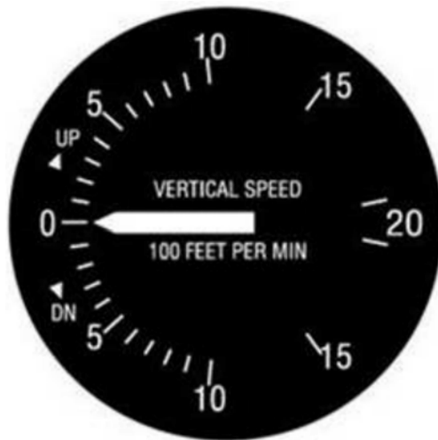
Figure 17B-3 Vertical Speed Indicator Parts
