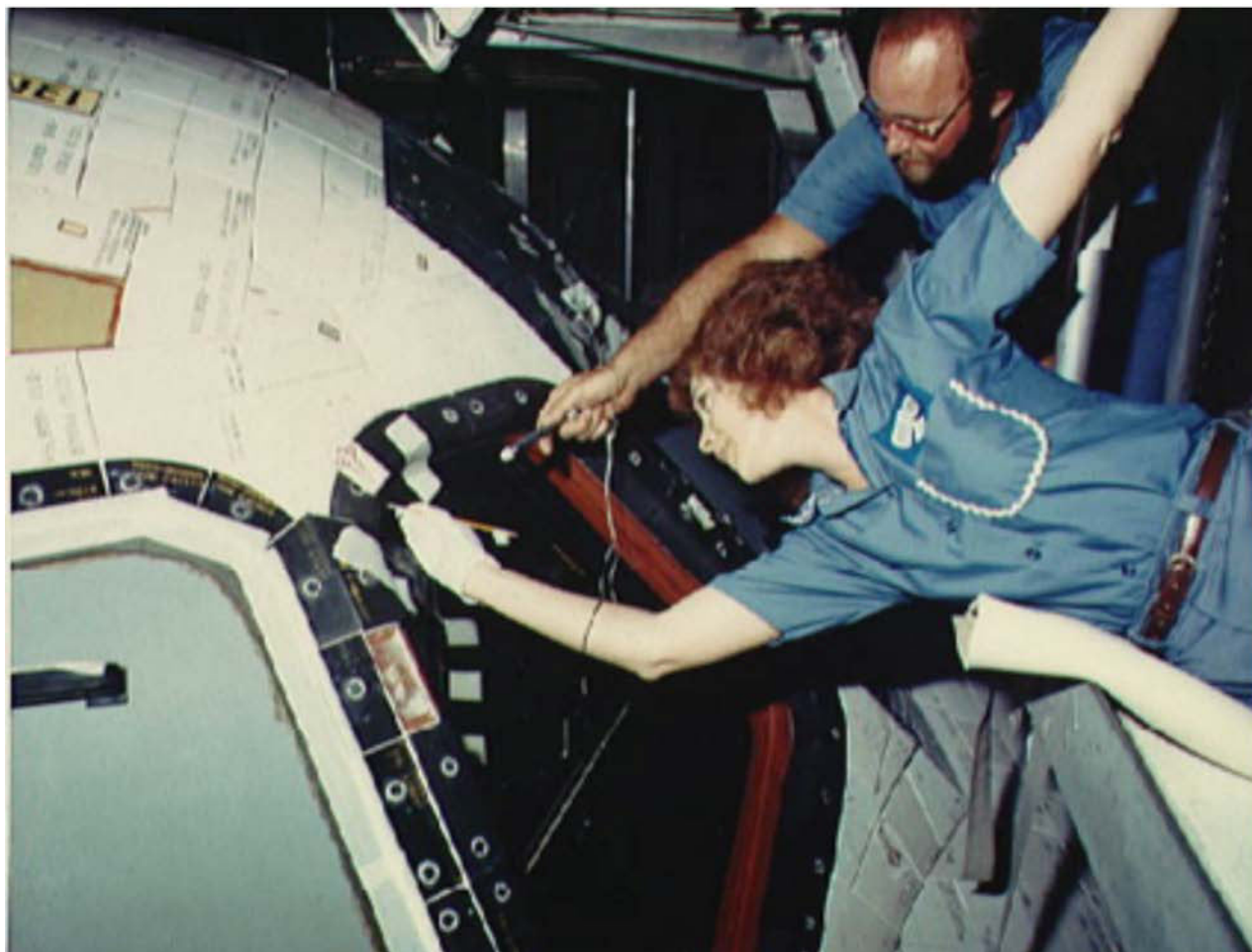
Figure 17O-4 Repairing TPS on Columbia
