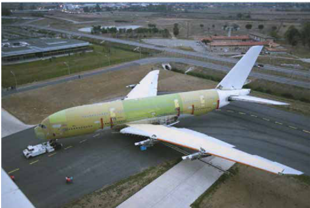
Figure B-4 Empty Pylons
