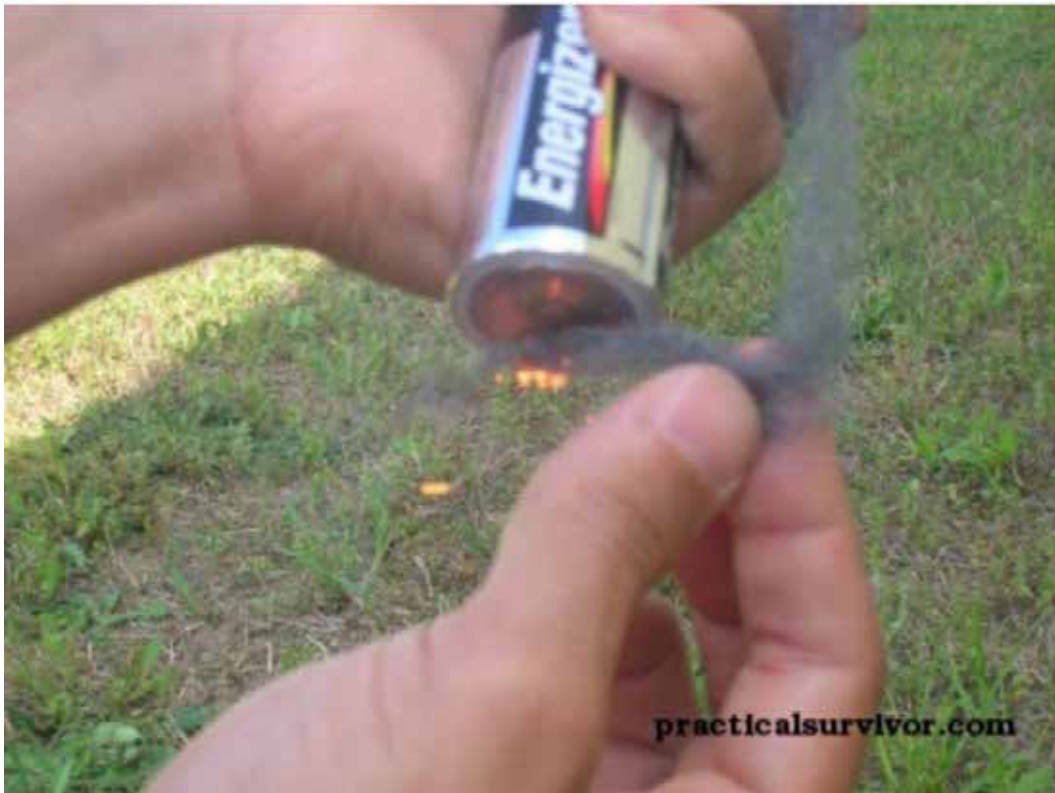
Figure 11 Battery and Steel Wool Ignition
