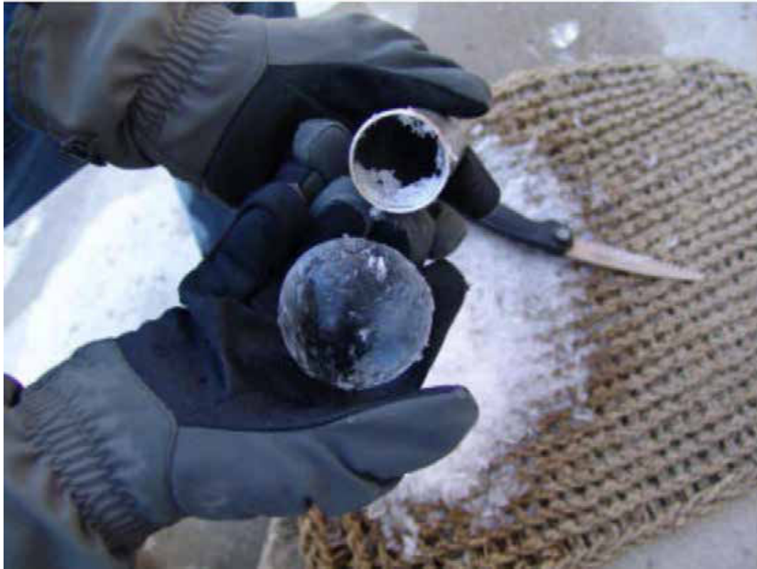
Figure 15 Using a Piece of Tubing to Shape an Ice Sphere
