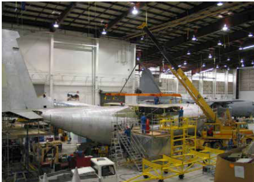
Figure A-2 Placing a C-130 Centre Wing
