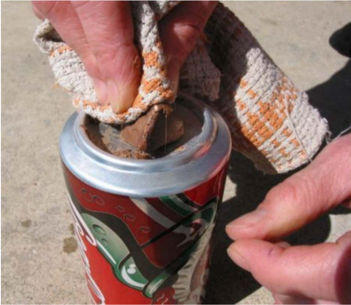
Figure 4 Polishing the Aluminum Can Bottom
