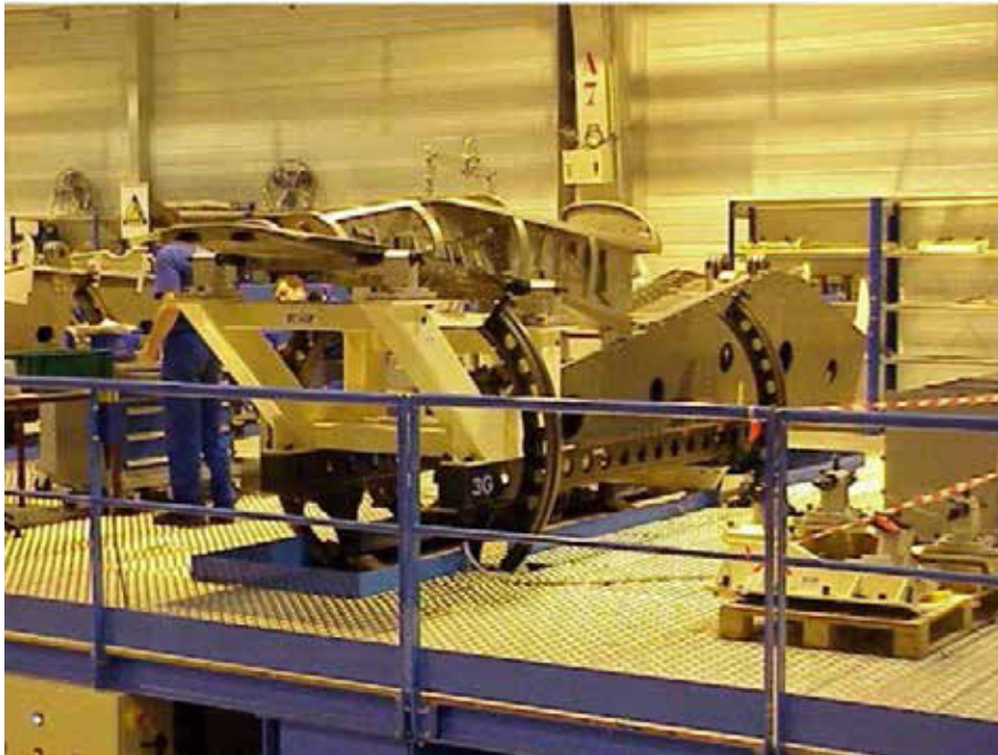
Figure B-1 Building a Pylon
