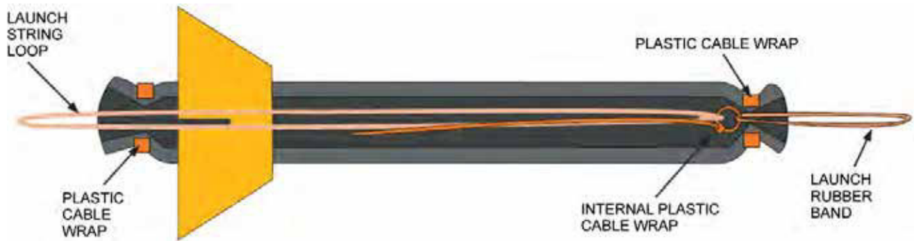
Figure 1 Exploded View of the Foam Rocket
