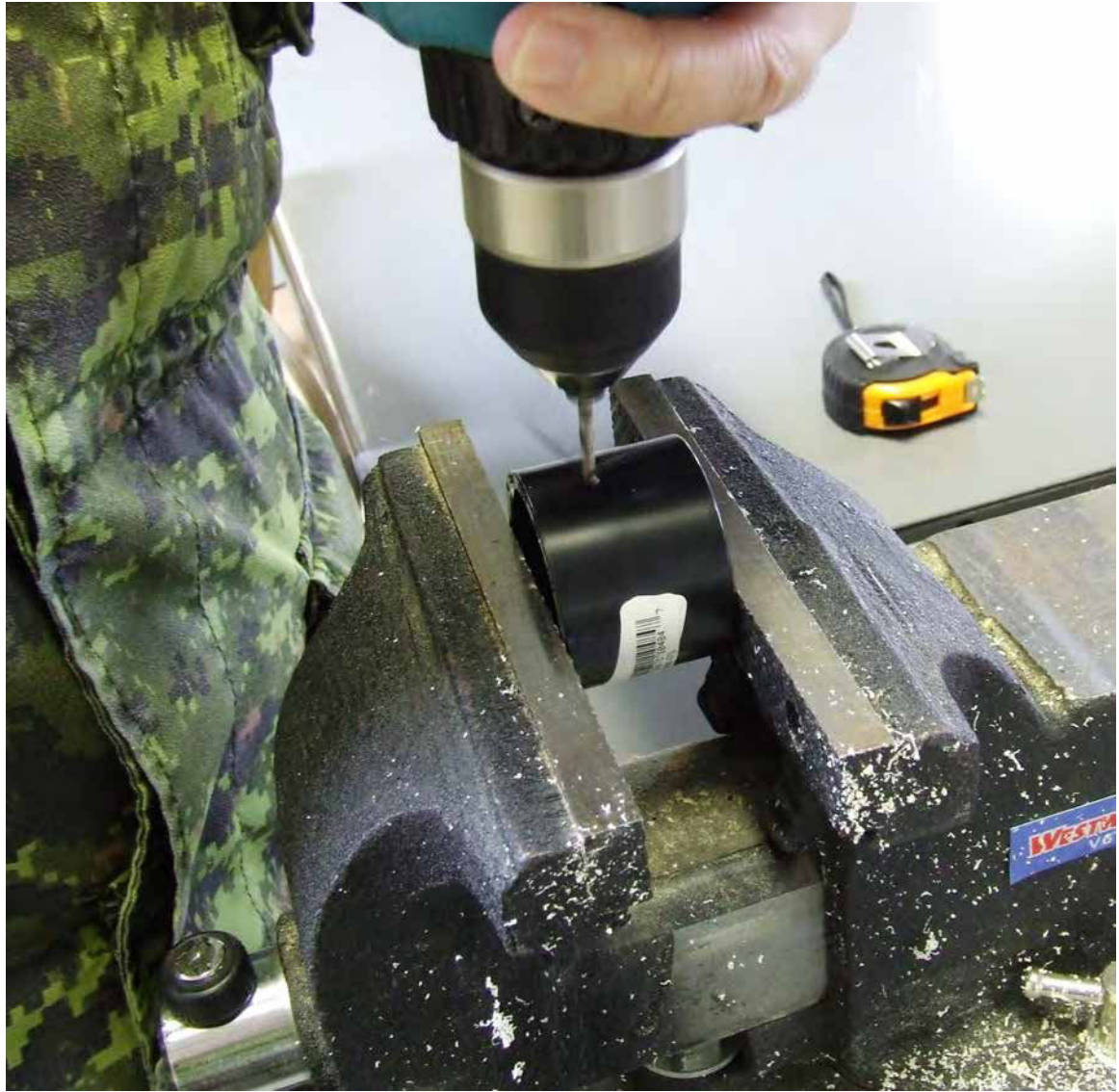
Figure 26-A Drilling 1/8-inch Holes in the ABS Coupler
